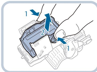
1. Squeeze the arrow indicated in step 3 (and its twin on the opposite side) to release the empty staple cartridge.
