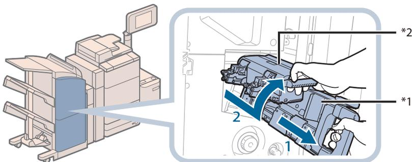
1. Grip the handle of the saddle sticher unit, and pull out until it stops.
