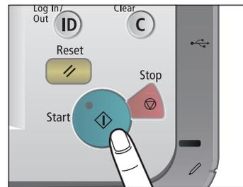
If the following screen appears, press **Start** (Start) to scan the next original. After all of the originals are scanned, press [Start Copying].
