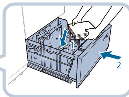
1. Load the paper stack against the left wall of the paper deck.
