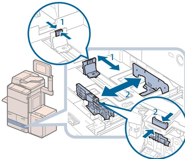
1. Slide the left guide while squeezing it on the top to align it with the mark for the desired paper size.
