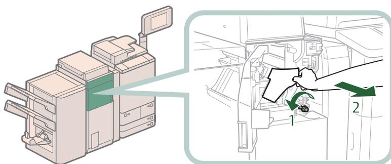
1. Turn the dial (M-A3) in the direction of the arrow (counterclockwise).
