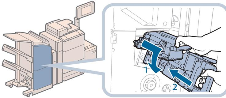
1. Pull the stapler unit of the saddle sticher unit towards you, and then push it down into its original position.
