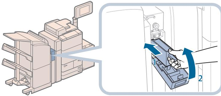
1. Push the punch waste tray back into its original position.
