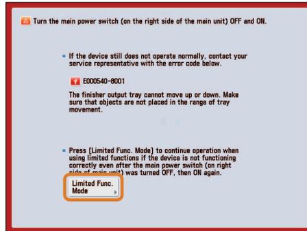
If [Limited Functions Mode] is displayed, you can temporarily set the Limited Functions Mode to continue to use the machine until the cause of the malfunction is cleared. For more information, see “Setting the Limited Functions Mode from the Service Call Message Screen,” on p. 262.
