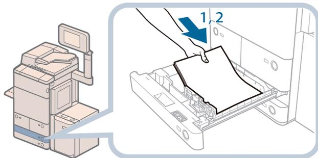
1. Make sure that the paper size setting of the paper drawer matches the size of the paper to load in the paper drawer.
