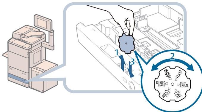
1. Open the inside cover of the paper drawer, and lift up the plate.
