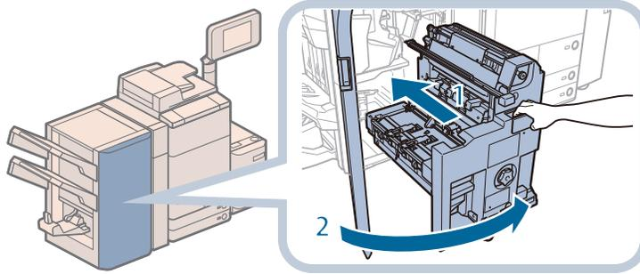
1. Gently push the saddle stitcher unit (F-C5) back into the machine. Always make sure to push the saddle stitcher unit in as far as it can go.
