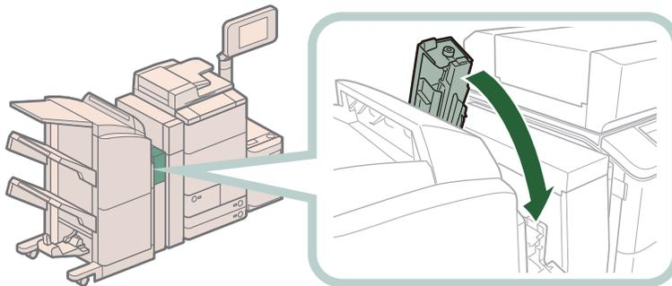
If you opened the insertion unit in step 2, gently push down the insertion unit back into its original position.
