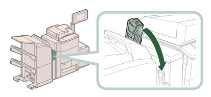
If you opened the insertion unit in step 2, gently push down the insertion unit back into its original position.
