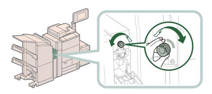
If the Document Insertion/Folding Unit-G1 or Document Insertion Unit-J1 is attached, open the insertion unit.
