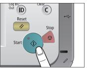
If the following screen appears, press ① (Start) to scan the next original. After all of the originals are scanned, press [Start Sending].
