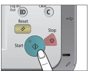
If the following screen appears, press ① (Start) to scan the next original. After all of the originals are scanned, press [Start Storing].
