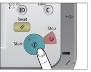
If the following screen appears, press  $\bigcirc$  (Start) to scan the next original. After all of the originals are scanned, press [Start Sending].
