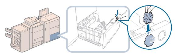
Gently push the paper deck back into the machine until it clicks into place in the closed position.
