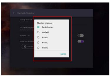
• For **OPS startup option**, you can choose **Startup only through OPS startup option** or **Startup through any channel**.
