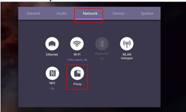
• Check the box of **Proxy Switch** to enable or disable the function.
