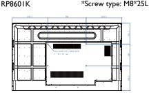
5. Install the wall mounting bracket on the display and attach the display to the wall according to the mounting bracket's instructions. The length of the screw should exceed the thickness of the wall mounting bracket by at least 25 mm. Make sure that all screws are tightened and secured properly. (Recommended torque: 470 - 635N•cm). The mounting means should be strong enough to bear the weight of the display.
